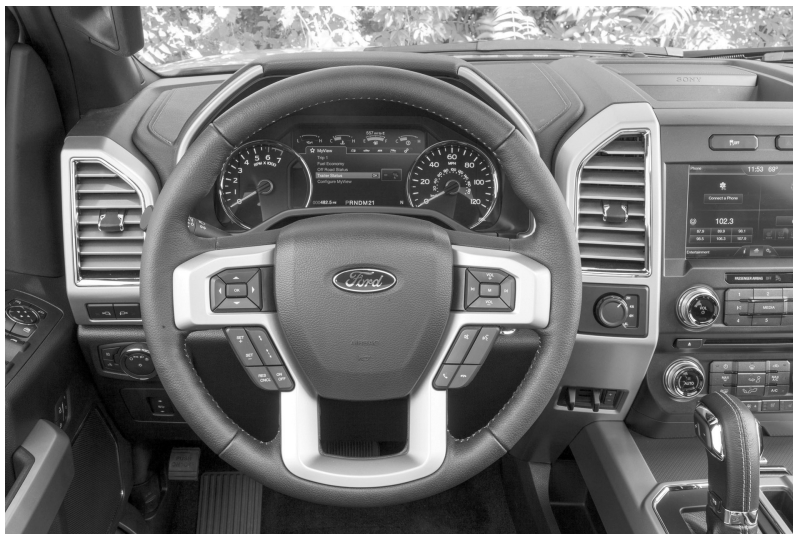
F-150's traditional, four-spoke design allows for a comfortable grip on the lower portion of the steering wheel. Other pickup truck manufacturers have closed off the bottom portion of the steering wheel. IMAGE COPYRIGHT FORD MOTOR COMPANY
